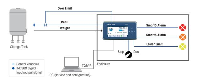
Stand-alone setup without PLC connectivity. IND360 controls refill valve and provides visualization on HMI. Start application with hardware switch attached to digital input of IND360. The "Over Limit Alarm" signal is attached to a safety switch acting as an emergency stop for refill. Configuration through web interface or display.
