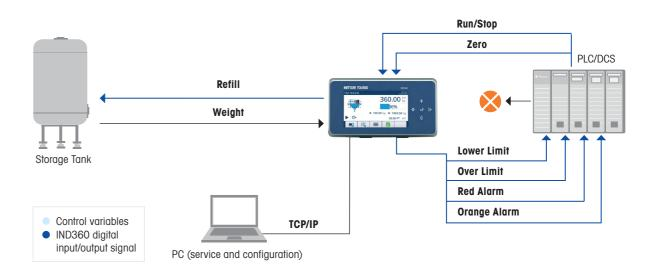
IND360 controls the refill valve and provides visualization on HMI. PLC access to status information and control functionality using digital I/O. Optional 4-20 mA weight output available for PLC/DCS connectivity. Configuration through web interface or display.
