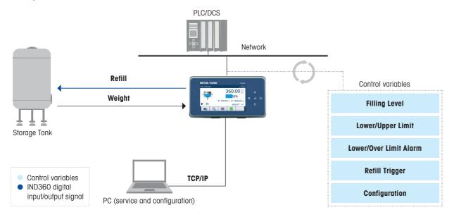
IND360 controls the refill valve while providing visualization on HMI. Cyclic and acyclic access to application status information and read/write of configuration using PLC interface, display or web interface. Redundant ring topology for PROFINET and EtherNet/IP is supported.
