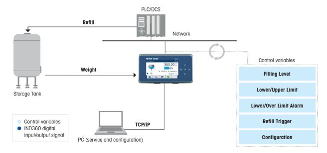
PLC controls the refill valve based on IND360 refill signal and other control information, the IND360 monitors the filling level and provides visualization on HMI. Cyclic and acyclic access to application status information and read/write of configuration using PLC interface, display or web interface. Redundant ring topology for PROFINET and EtherNet/IP is supported.
