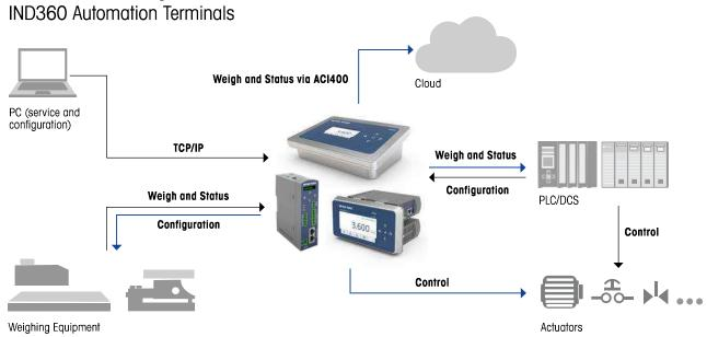
IND360 connects many different types of weighing equipment to automation controls such as PLCs or DCSs. It provides the ability to manage weighing applications that directly drive outputs for actuators and receive inputs from switches - see IND360 manuals for more details. IND360 is very easy to setup using the web interface that is accessed via a web browser such as Microsoft Edge or Google Chrome. When cloud connectivity is desired, choose the METTLER TOLEDO ACI400.
